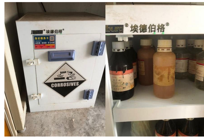
危化品柜未上锁, 试剂标签已腐蚀
